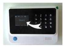
1. Make sure your alarm system is disabled to avoid a false alarm trigger when you are changing the battery in the sensor.
