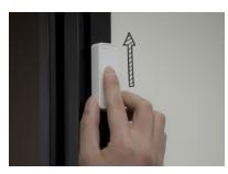
2. Push the door sensor up to remove it from the frame
