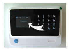
1. Make sure your system is disarmed to avoid a false alarm trigger when you are changing the batteries in the sensors.
